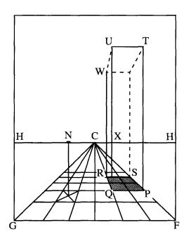
Figure 13 Examples of the construction of scaled forms on the 'pavement' O: A distance of 1 i/2 braccia into the picture, determined by the diagonals of a square in the second row. ON=3 Braccia. PQRS: Plan of rectangular object on a base 2 braccia square. QX= 3 baccia. QU= 9 braccia (note: Alberti's example is a further 3 braccia high). TUW: top of the visible faces of the object (all other labels as in Fig. 11).
