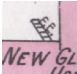
a fire escape
