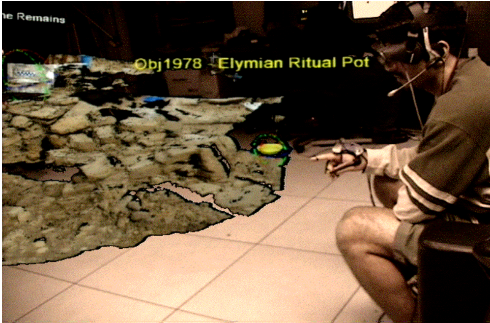
Figure AR-SYSTEM. User's view of a virtual representation of the Monte Polizzo site in augmented reality. Users wear head-tracked, see-through, head-worn displays. Objects, such as the labeled pot, are represented either with a 3D model or with a picture if the model is not available. This image was rendered in real time through another tracked camera representing a second user's view.
