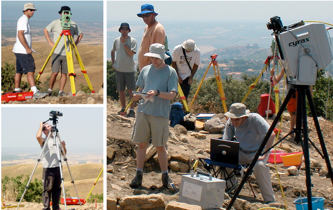
Figure MP: On top of Monte Polizzo: members of our team record exact 3D coordinates using a total station surveying instrument (upper left), capture video of an excavation using a digital camera (lower left), and scan a portion of the dig site using the Cyrax range scanner (right).
